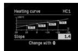
Example: Vitotronic 200 HO1B heating curve
