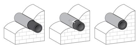
Remove the grid-cover from the grill by sliding it upwards. Screw the grid to the outside wall using the 4 plug screws 4 x 40 mm (supplied with the unit). Re-mount the grid-cover sliding it down along the outside grill.
