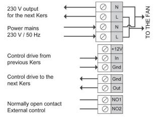
To power the devices (230V single phase 50 Hz) use used copper wires with a section between 0.5 mm<sup>2</sup> and 0.75 mm<sup>2</sup>. For the control wiring, a shielded 0,25 mm<sup>2</sup> will be enough.
