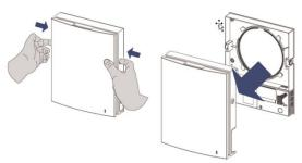
Fix the rear part of the unit against the wall with the supplied screws. Open the transparent cover to connect the DC power cable to the terminals according to the wiring electric diagram.
