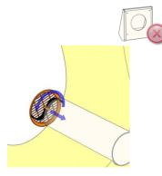
Without removing the protective paper, roll up the insulation and place it once within the duct up to the stop. Measure the distance that separates the insulation from the entrance of the duct: must be at least 28 cm. If it were lower, pull out the insulation and cut off excess. Reinsert the insulation into the duct. Insert the main body of the unit until it stops, without pushing off the arid.
