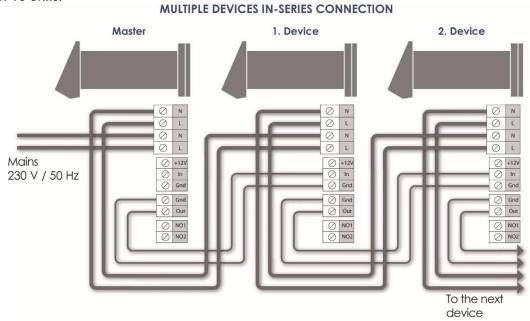
The first unit KERS (master) controls all the others. The units must be set in a way that half of them begin their cycle in extraction, and the other half in supply phase, this way the rooms will not be subject to air pressure imbalances. A series of dip-switch, located under the rubber end cap, allows to set such phases. (See chapter "setting DIP-switch").
