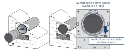
Install the front panel taking care that the actuator pin completely retracted at the bottom, to prevent any damage to it.
