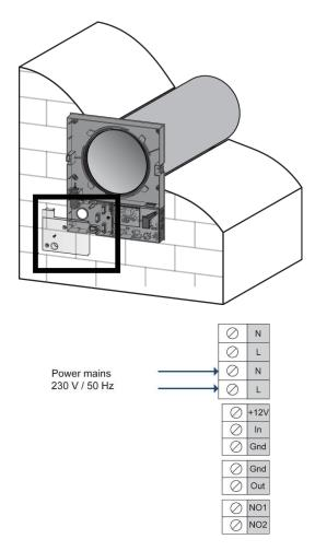
The unit is built to work with AC single-phase 230 V/50 Hz.
